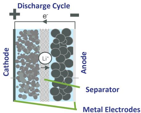
Today's Li ion batteries use graphite as active anode material. Silicon - with its higher specific capacity - will enable the next generation of Li ion batteries for electric vehicles.
